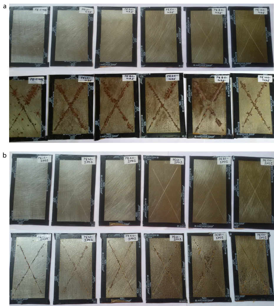
Fig. 9 Salt spray test panels of (a) PE-N75 (0, 500 h), (b) PE-IPDI system (0, 500 h).
